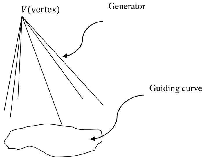
A cone which is represented by an equation of second degree is called a **quadratic** (or **quadric**) cone. Any straight line other than the generators intersects a quadric cone in two points.
