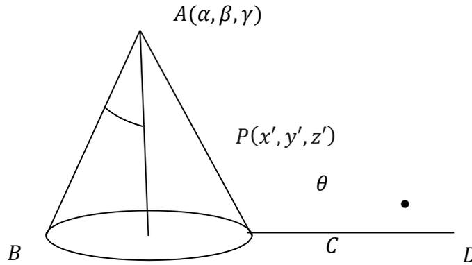
Let  $P(x', y', z')$  be any point on the surface of the cone. Then the direction cosines of the line  $AP$  are proportional to  $x' - \alpha, y' - \beta, z' - \gamma$ . If  $\theta$  is the semi-vertical angle of the cone, then we have
