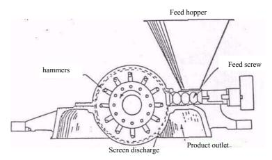
Figure 9.5: Sectional view of hammer mill
