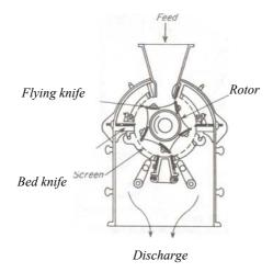
Figure 5.10: Rotary knife cutter
