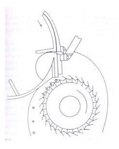
Figure 6.1: Slicing equipment
