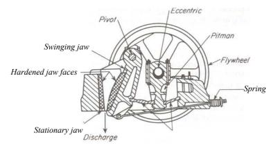
Figure 5.1: Jaw crusher
