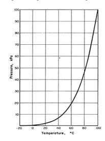
Figure 1.21: Phase diagram for water
