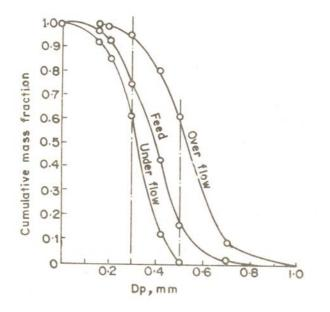
Figure 3.10: Graphical representation of various flows of a screen
