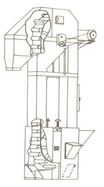
Figure 7.8: Bucket elevator
