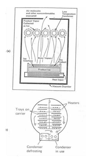
Figure 12.15: Freeze drying: a) Schematic illustration of freeze drying system; b) Crosssectional view of a continuous freeze drier.
