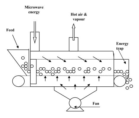
Figure 12.13: Schematic of a continuous microwave drying equipment
