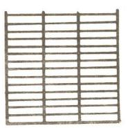
Figure 3.17: Wire mesh screen (square openings)
