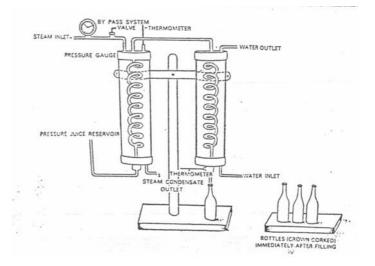
Figure 9.10: Schematic representation of a flash pasteurizer
