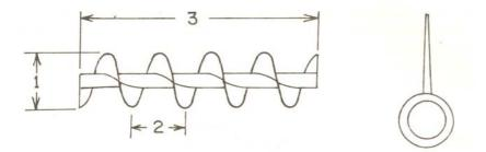
Figure 7.3b: Screw conveyor-details: 1) Screw diameter, 2) Pitch of screw, 3) Screw length
