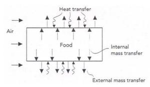
Figure 1.20: Principle of drying of food
