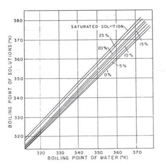
Figure 1.12: Duhring lines for sodium chloride – water system
