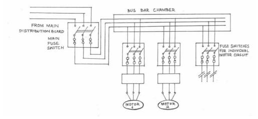
Figure 14.1: Supply from busbar chamber to individual machines
