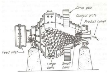
Figure 5.8: Conical ball mill
