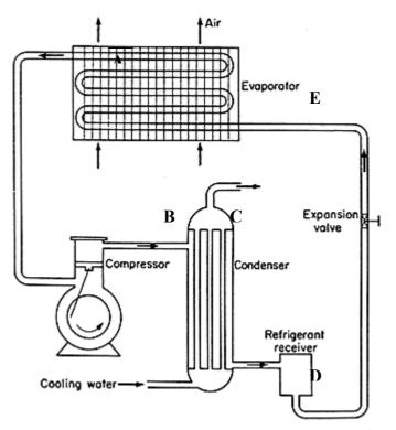
Figure 1.6: Mechanical refrigeration circuit
