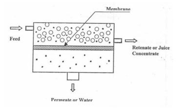
Figure 9.12: Schematic representation of ultrafiltration process
