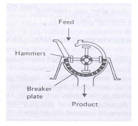
Figure 6.5: Hammer mill
