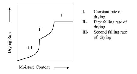
Figure 12.2: Moisture content vs. drying rate
