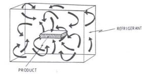
Figure 1.11: Schematic diagram of direct contact freezing
