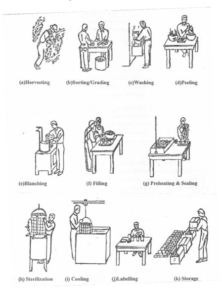
Figure 11.7: Schematic representation of fruit canning unit operations
