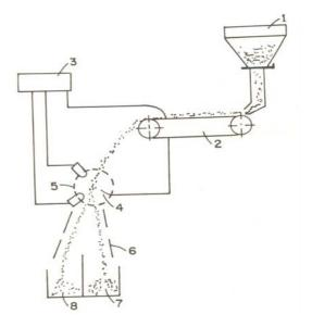
Figure 3.7: Schematic of a colour separator 1) hopper, 2) belt conveyor, 3) amplifier,
