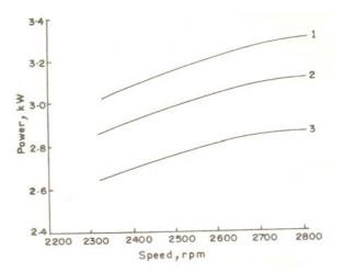
Figure 6.10: Effect of speed of operation on power requirement: 1) 17.9% moisture content, 2) 15% moisture content, 3) 11.8% moisture content.
