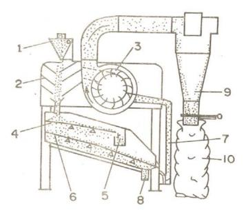
Figure 3.2: Schematic diagram of a vibratory air screen cleaner. 1) Feed Hopper,
