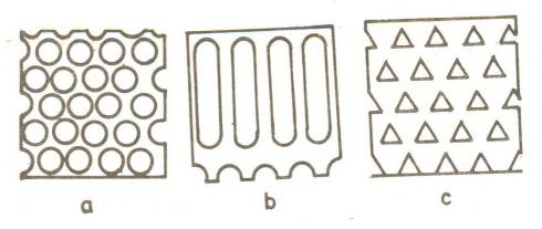
Figure 3.16: Perforated metal screens. a) Round holes, b) Oblong holes, c) Triangular holes
