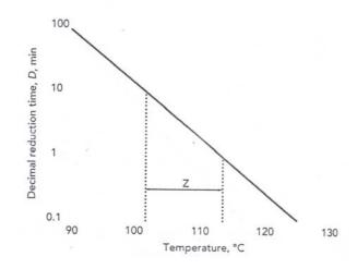
Figure 1.4: Thermal resistance curve of microbial population
