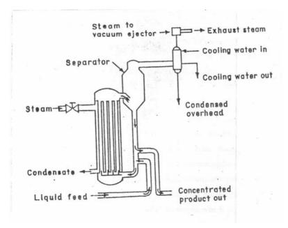
Figure 9.11: Diagram of a typical evaporator
