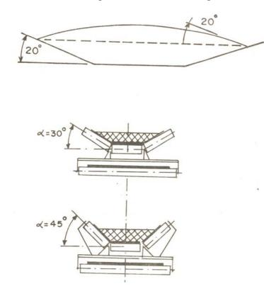
Figure 7.2: Various troughing configurations
