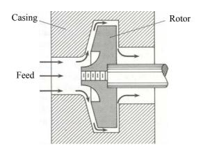
Figure 5.9: Schematic drawing of colloid mill
