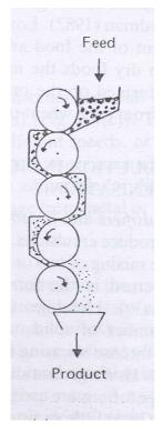
Figure 6.6: Roller mill
