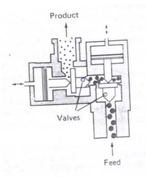
Figure 6.7: Hydraulic two-stage pressure homogenizing valve
