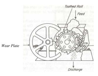
Figure 5.4: Single-roll tooth crusher
