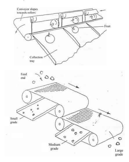
Figure 9.3: Sorting machines: a) Belt and roller sorter; b) Screen grader
