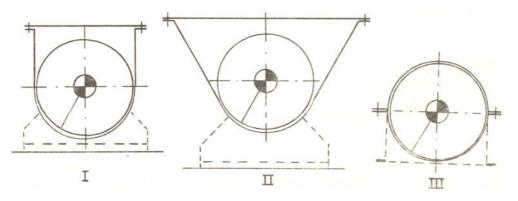
Figure 7.4: Various shapes of screw conveyor trough I) U-trough, II) Flared trough, III) Tubular trough.
