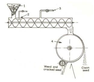
Figure 3.8: Magnetic Separator. 1) Feed hopper, 2) Water spray, 3) Iron powder mixing, 4) Magnetic drum.
