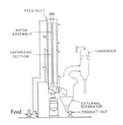
Figure 1.19: Agitated thin film evaporator
