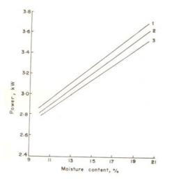
Figure 6.9: Effect of moisture content on power requirement: 1) 2800 rpm, 2) 2680 rpm, 3) 2560 rpm.
