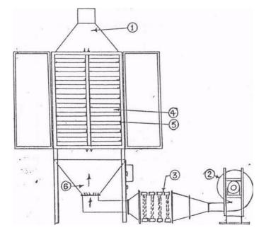
Figure 12.7: Schematic diagram of a typical tray drier: 1) Exit air, 2) Blower, 3) Heater, 4) Inter space between trays, 5) Trays, and 6) Plenum chamber
