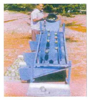
Figure 3.6: Size based mango grader
