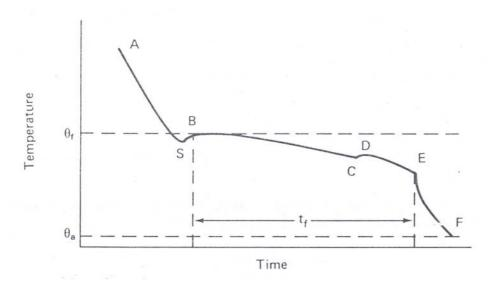
Figure 1.8: Time temperature relationships during freezing
