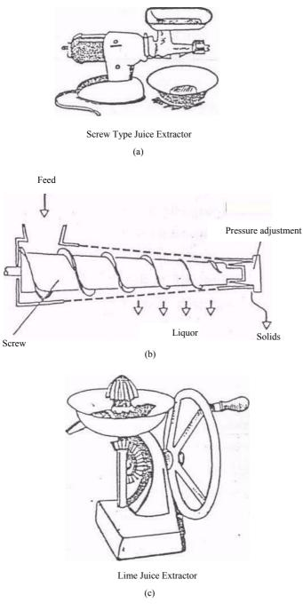
Figure 9.6: a) Screw extractor; b) Working principle of screw press; and c) Lime juice extractor
