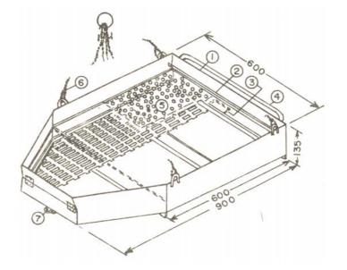
Figure 3.1: Hand operated double screen grain cleaner. 1) frame 2) draper rod 3) screen handle 4) handle 5) scalper and grader screens 6) rope attachment 7) shutter opening attachment
