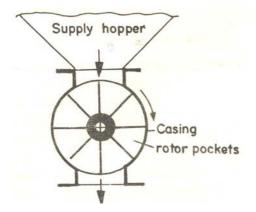
Figure 7.6: Rotary feeder for pneumatic conveyor
