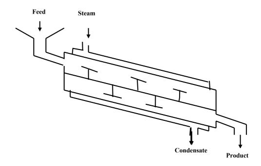
Figure 12.14: Rotary dryer
