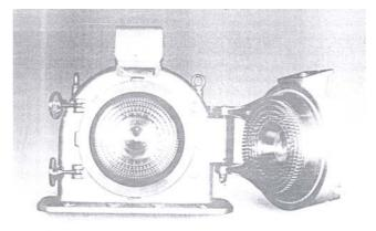
Figure 6.4: Pin and disc mill
