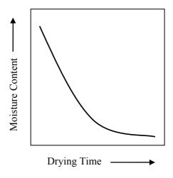
Figure 12.3: Drying time vs. moisture content
