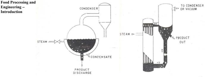
Figure 1.13: Batch type pan evaporator
