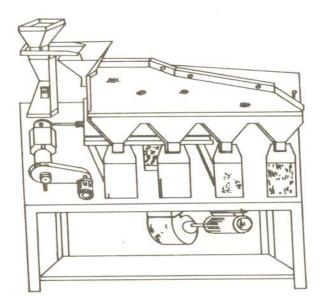
Figure 3.4: Specific gravity separator
