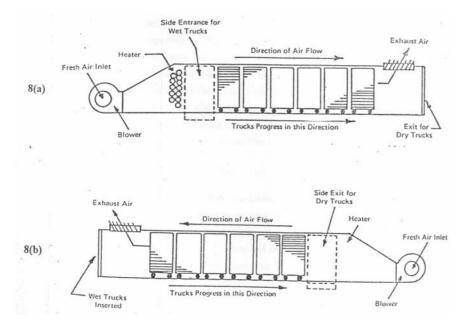
Figure 12.8: Schematic of tunnel driers: a) Concurrent flow drier, b) Counter-current flow drier
