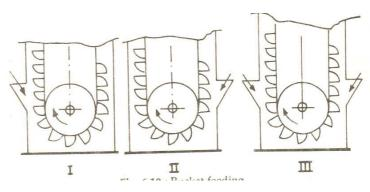
Figure 7.9: Bucket feeding I) Front feed, II) Back feed, III) Combined feed.
