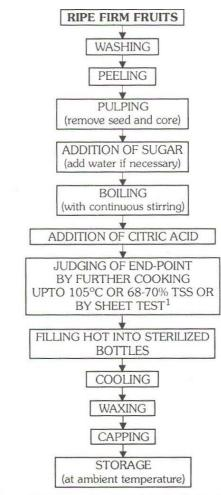
1. Sheet or flake test: A small portion of jam is taken out during boiling, in a spoon or wooden ladle and cooled slightly. It is then allowed to drop. If the product falls off in the form of a sheet or flakes instead of flowing in a continuous stream or syrup, it means that the end-point has been reached and the product is ready, otherwise, boiling is continued till the sheet test is positive.
