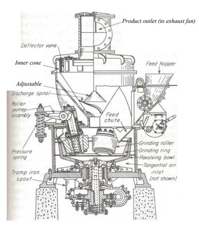
Figure 5.6: Roller mill
