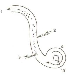
Figure 3.5: Diagram of a pneumatic separator. 1) Undersirable material removal, 2) Uniform feeder, 3) Clean grain outlet, 4) Centrifugal blower, 5) Control for air intake
