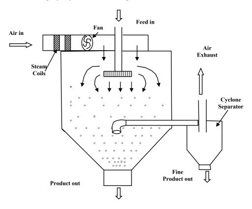
Figure 12.12: Typical schematic arrangement of a spray dryer
