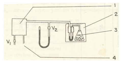
Figure 2.2: Schematic diagram of an isotenoscope: 1) Vacuum storage jar, 2) Constant temperature water bath, 3) Sample flask and 4) Vacuum pump
