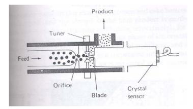
Figure 6.8: Ultrasonic homogenizer
